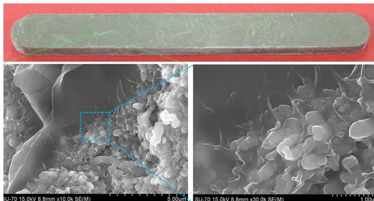
Figure1: Photograph of nanocomposite specimen prepared with 0.5 wt% of GO. SEM images show a good integration of the fillers with the polymer.
