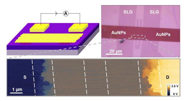
Top: Schematic and optical image of graphene contacted device. Bottom: KFM image of the nanoparticle network region shown in the optical image. In addition to the outer source and drain, an equipotential floating graphene structure flattens the potential landscape in the middle three sections.
